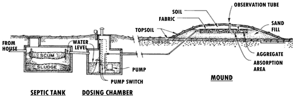
From the septic tank, the wastewater typically passes into a dosing chamber (pump chamber). This is another tank which collects the effluent and contains a pump which uses pressure to evenly distribute the wastewater into a distribution system in the sand mound. The dosing chamber and pump typically are connected to an alarm which alerts you to any malfunction or problem with the dosing system.
