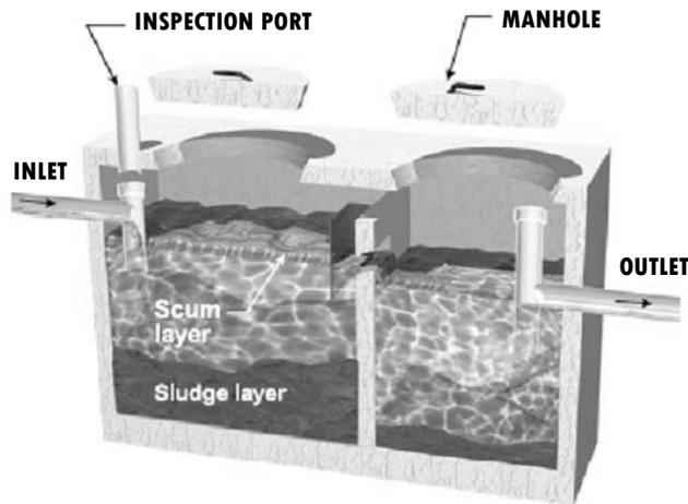
If the tank is not periodically pumped out, these solids will eventually clog the pipes and/or soil pores in the absorption (leach) field to the point where a new sand mound will be needed.
